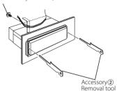
4 Push upward the removal tool toward the top, and pull out the unit halfway while pressing towards the inside.
